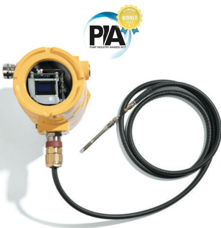
“The ultrasonic condition monitoring instrument is proving even more useful than we thought,” commented the Senior Process Engineer. For example, he explained that, when the process is coming back on stream, the liquid entering the pump is unstable for a period of time. By having visibility of conditions inside the pump, the user can avoid premature start-up (which could damage the pump) and ensure that the pump is brought on-line as quickly as possible – maximising productivity.
