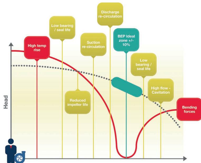
Figure 7 Operating outside the best efficiency point (BEP)
